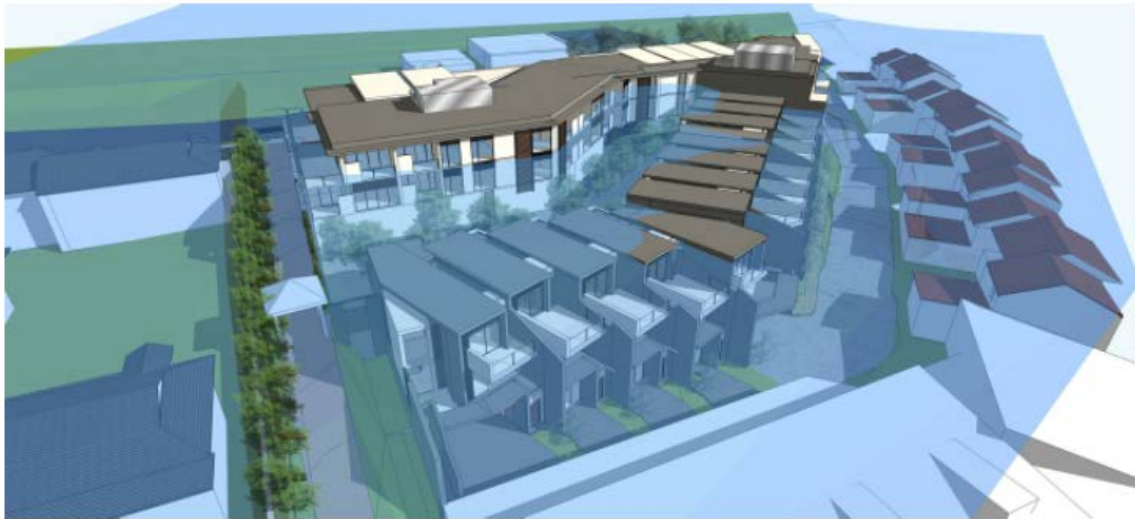
HEIGHT PERSPECTIVE 1 (IMAGE ABOVE DISPLAYING BUILDING ELEMENTS OVER THE 9m HEIGHT LIMIT RELATIVE TO NATURAL GROUND LINE)
